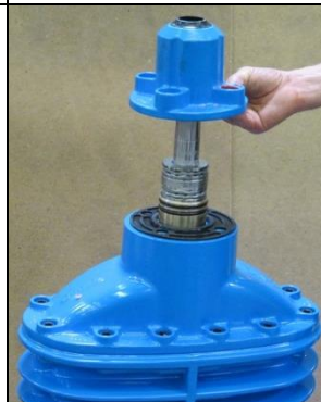
4. In case the upper ball bearing or the bearing ring remains in the central flange, take them out.
