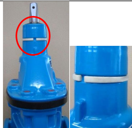
2. Place the retaining ring into the slot. The gap in the retaining ring and the locking rib have to be aligned.
