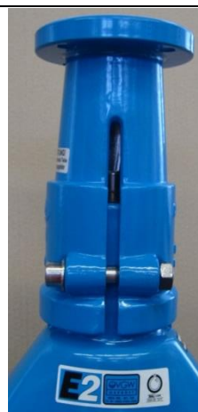
6. Attach the lantern to the upper body with the included bolts. Maximum tightening torque: 80Nm
