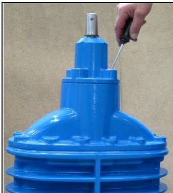
1. Remove the wax sealing from the centering flange screws.
