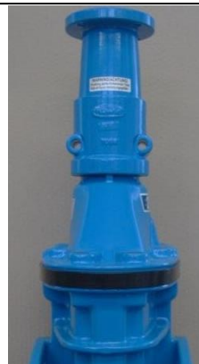
4. Mount the lantern onto the upper body, all the way to the end stop.
