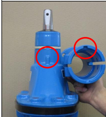
3. Mount the lantern on the upper body. The locking rib and the recess in the lantern define the mounting position.
