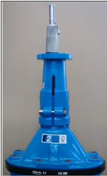
7. Attach the spindle socket and the spigot onto the spindle in the lantern.
