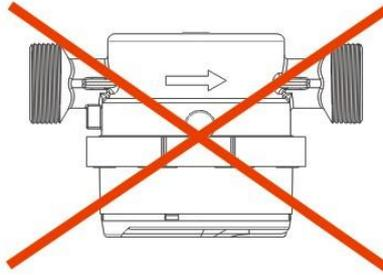
Rys. 2. Prohibited installation positions of water meters manufactured by Apator Powogaz SA, type JS (DN 15-40).
