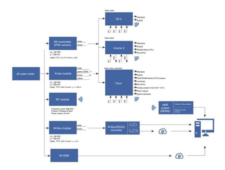
Rys. 5. Diagram of example connections for the implementation of remote indication transmission.
