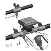
Length of connecting cable for flow rate sensor/unit: 0.5 m
