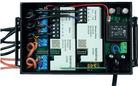
Wireless M-Bus-module with internal antenna
