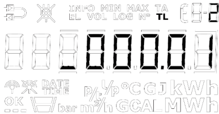
Figure 21 - Setting up positive TL2 in "SETUP loop", the _ will be flashing when on the sign position but disappear when moving to another decimal.
