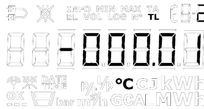
Figure 22 - Setting up negative TL2 in "SETUP loop", the - will be flashing when on the sign position and stay on when moving to another decimal.
