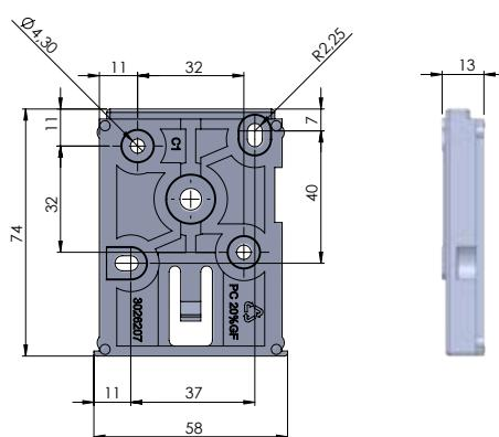
**Calculator base separate and mounted on ULTRAFLOW®**
