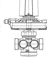
Since all differential pressure controllers of the 4002 and 4202 series have a pressure relieved upper part, these automatic zone valves can also be
