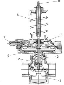
Ammonia contained in hemp damages brass valve housings, EPDM seals are swollen by mineral oils or lubricants containing mineral oils and thus lead to failure of the EPDM seals. For antifreeze and corrosion protection agents based on ethylene
