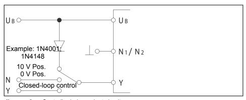
diagram 9 Controller independent circuit
