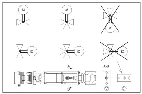
diagram 5 Assembly positions for linear actuator and valve
