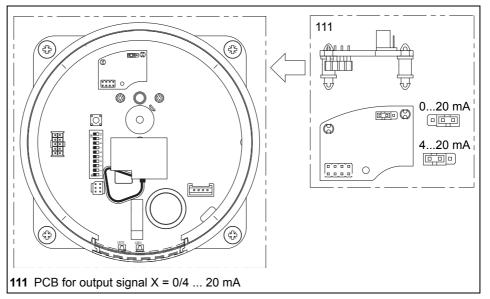
diagram 2 PCB for mA output signal in cover
