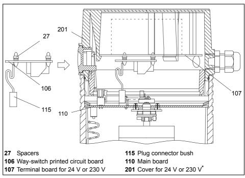
diagram 10 Installation of the way-switch printed circuit board in the cover
