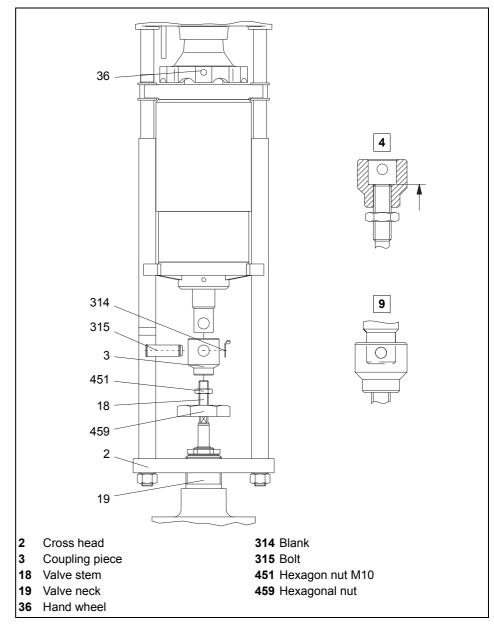
diagram 6 Mounting the linear actuator on the valve
