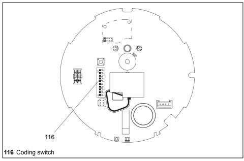
diagram 14 Printed circuit board cover and coding switches
