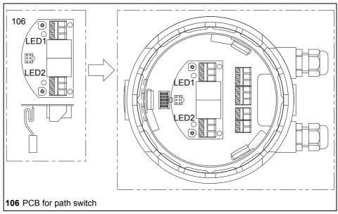
diagram 3 Position switch PCB in cover
