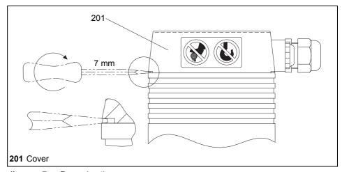
diagram 7 Removing the cover
