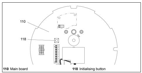
diagram 19 Initialising the path measuring system
