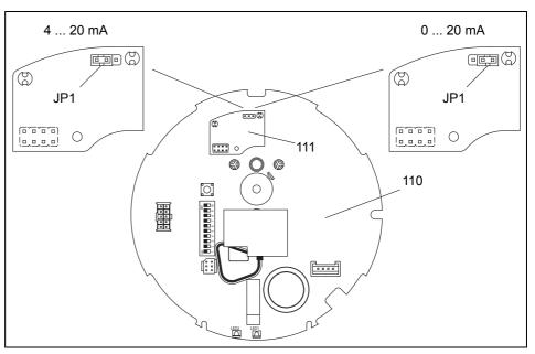
diagram 13 Set signal range for mA output signal X
