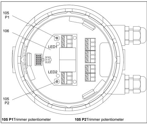
diagram 18 Way-switch printed circuit board in cover
