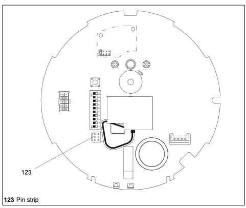
diagram 11 Pin strip for way-switch printed circuit board on the motherboard
