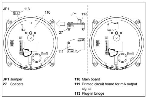
diagram 12 Installation of the printed circuit board for mA output signal
