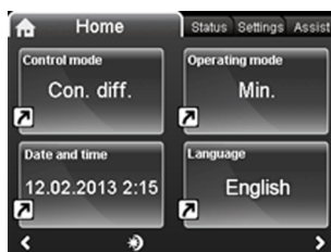
Example of main display on a TPE Series 2000 with advanced control panel
