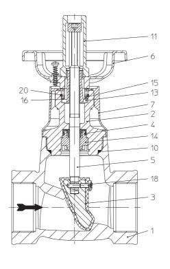
Fig. 3: EURO-WEDI length FTF-14 screwed socket connection
