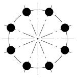
DN 65 PN 10/16 (steel/steel): DIN EN 1092-1 with DIN EN 1092-1: Bolts through 8 holes
