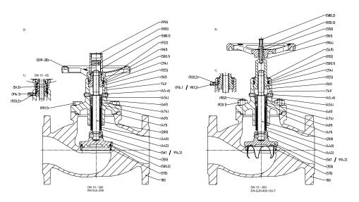
**Fig. 23:** Sectional drawings; 1) shown rotated by 90°; 2) variant with PTFE ring on valve disc; 3) variant with V-port plug
