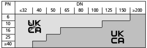
Fig. 5: UKCA marking: BOA-SuperCompact, BOA-Compact, BOA-Compact EKB, BOA-W and BOA-RVK
