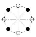
DN 65 PN 10/16 (steel/cast iron): DIN EN 1092-1 with DIN EN 1092-2: Bolt hole circle to DIN EN 1092-1 turned through 22.5°, bolts through 4 holes, 4 holes free
