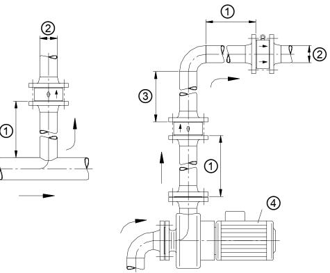
Fig. 16: Minimum upstream stabilisation distances
