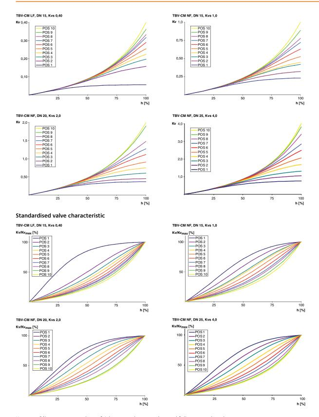
$Kv_{max} = m^3/h$  at a pressure drop of 1 bar at each pre-setting and fully open valve plug.  $Kvs = m^3/h$  at a pressure drop of 1 bar and fully open valve. h = lift
