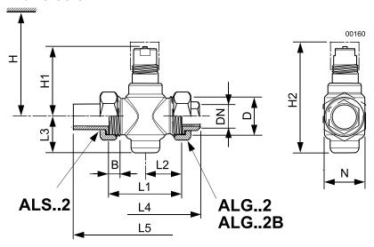
H(\*) = Total height of actuator plus minimum mounting distance to wall or ceiling, for mounting, connection, operation, maintenance, etc.
