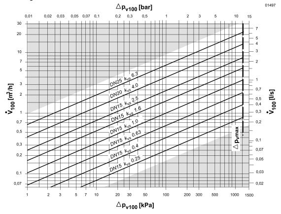
$\Delta p_{\text{max}}$  = Maximum permissible differential pressure over the valve control path, valid for the entire positioning range of the valve-actuator unit:
