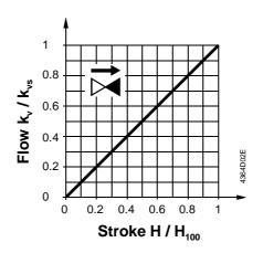
Valve flow characteristic linear as per VDI /VDE2173
