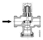
Guided parabolic plug which is integrated in the valve stem.
