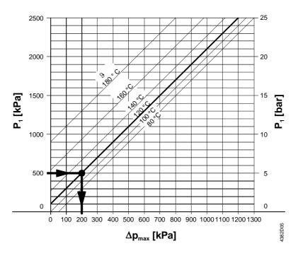
Differential pressure with valve almost closed, at which
