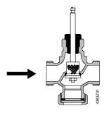
Guided perforated plug which is integrated in the valve stem.
