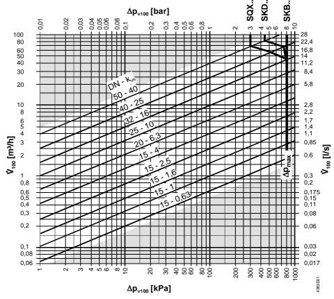
$\Delta p_{\text{max}}$  = Maximum permissible differential pressure across the valve, valid for the entire actuating range of the motorised valve
