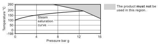
**Please note:** The figures displayed are only relevant when a metal-to-metal seat is used. If Viton or EPDM seats are used the product is restricted to the limits of the seat material chosen.
