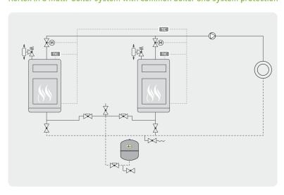
When the burner is switched off, the final control element (in its closed by the temperature controller preventing incorrect circulation via the shut-off boiler. Joining the boiler expansion line above the centre of the boiler prevents gravity circulation. Preferred inset in systems without minimum boiler return flow temperature (e.g. condensing boiler systems).
