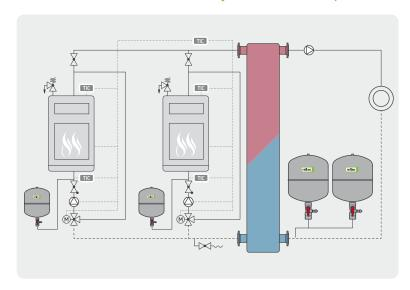
The serial circuit of several Reflex N 6 or 10 bar vessels generally produces economical alternatives to Reflex G large vessels.
