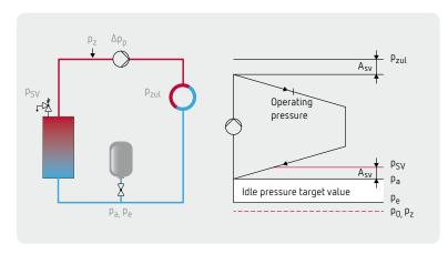
The pressure maintenance is integrated **upstream** of the flow-through pump, i.e. on the suction side. This method is used almost exclusively because it is the easiest to control.
