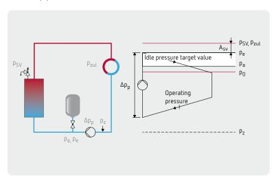
Pressure maintenance is integrated **downstream** of the flow-through pump, i.e. on the pressure side. When determining the idle pressure, a facility-specific differential pressure component for the flow-through pump (50...100%) must be included in the calculation. For use in only a limited number of cases  $\rightarrow$  solar systems.
