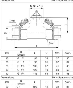
Dimensions "Hycocon HTZ" DN 20 k<sub>vs</sub> value 5.0 Item no. 1068667
