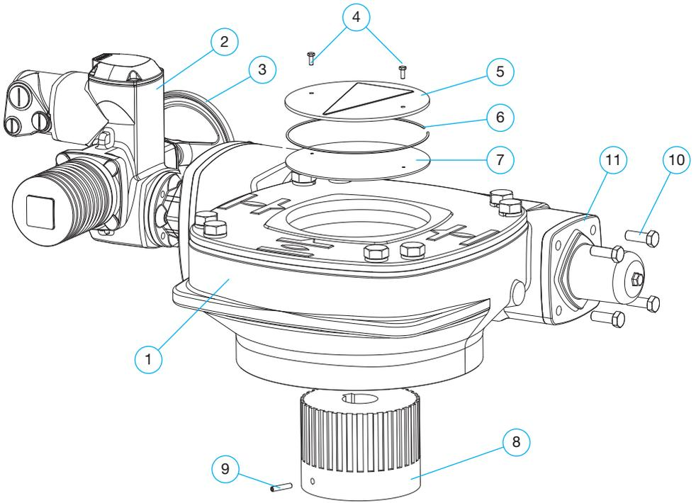
Figure 14. Electric actuator.
