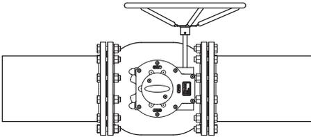
Figure 7. Horizontal installation.
