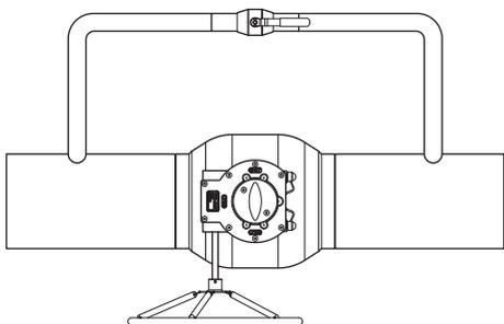
To avoid pressure shocks and to reduce the forces caused by opening the valve under pressure, it is recommended to use a by-pass valve in connection with ball valves of size DN 150 and larger (see Figure 11).
