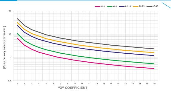
To make sizing easier, a chart has been drawn up to select the most appropriate accumulator according to both the working pressure and delivery criteria. Note that the chart is based on the following hypothesis: standard precharge and 15 pump starts per hour (see p. 27 to identify the "X" coefficient).
