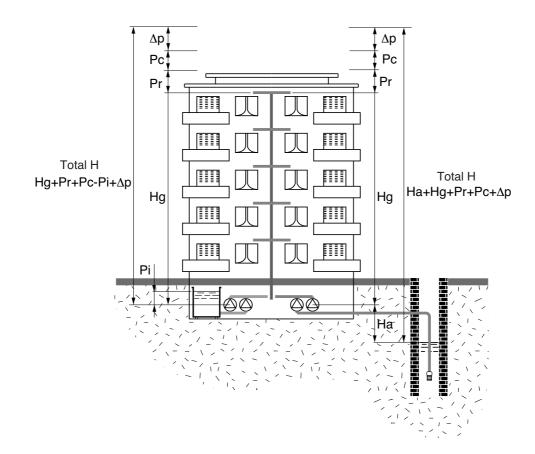
When the pumps draw water from a well, the dynamic height difference (Ha), when pumps are operating, should not exceed 4 m. A greater suction head or erroneous sizing of the suction pipe may cause improper operation of the pumps - e.g. cavitation and priming loss. The pumps are installed with a positive suction head when they are connected to a raised tank or a pressurized primary collection tank.
